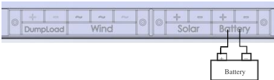
Battery wiring(the positive and negative cannot be reversed)
